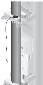
Placement on a Sector Antenna
