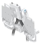
a. For most antenna models, the airFiber NxN Multiplexer should be installed at a 15° angle. Insert the airFiber NxN Multiplexer from behind the 4x4 Radio Bracket and slide the 15° Angle Tabs into the slots on the bracket.
