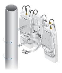
Connect the RF cables from the antenna to the RF connectors on the airFiber NxN Multiplexer. Connect +45° to Chain 0 and -45° to Chain 1.
