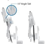
b. For other antenna configurations that require the airFiber NxN assembly to be mounted to a pole, the airFiber NxN Multiplexer must be installed vertically. Insert the airFiber NxN Multiplexer from behind the 4x4 Radio Bracket and slide the Vertical Tabs into the slots on the bracket.
