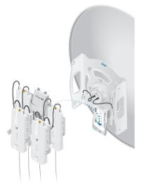
Note: The airFiber NxN assembly may be pole-mounted if it cannot be attached to the antenna. See the Pole-Mounting section for details.  Connect the RF cables from the antenna to the RF connectors on the airFiber NxN Multiplexer. Connect +45° to Chain 0 and -45° to Chain 1.
