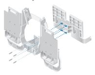
2. Seat the *airFiber NxN Multiplexer* into the *4x4 Radio Bracket* either at (a) a 15° angle or (b) vertically:
