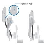
3. Secure the airFiber NxN Multiplexer to the 4x4 Radio Bracket using two M4x12 Screws.
