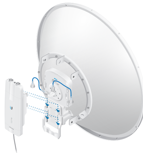
Mounting the AF-11FX on the AF-11G35
